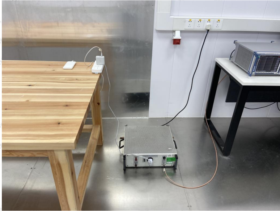
Photo of Power Line Conducted Emission Test
