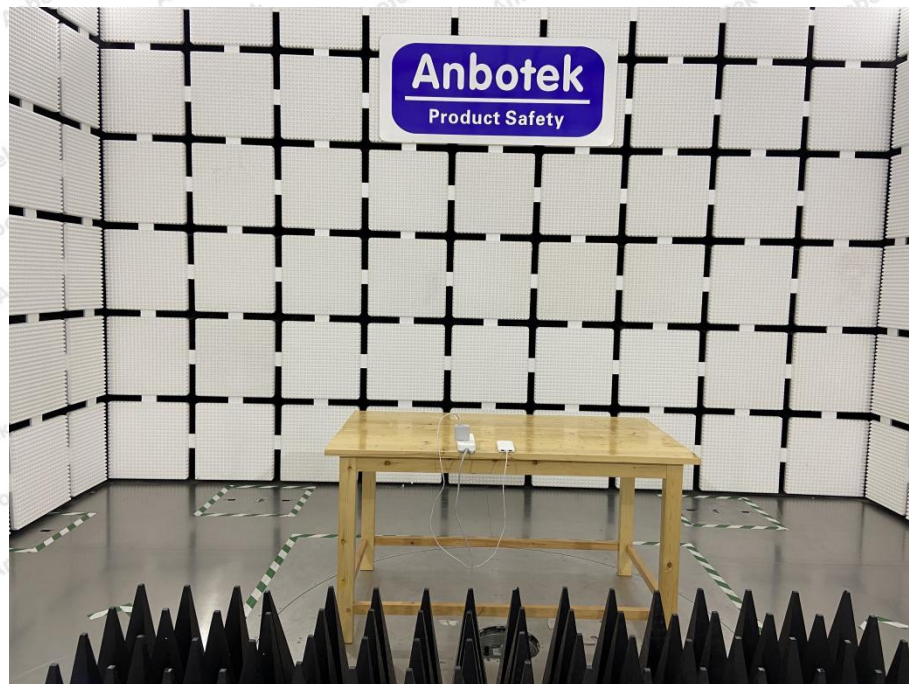
Photo of RF Field Strength susceptibility Test
